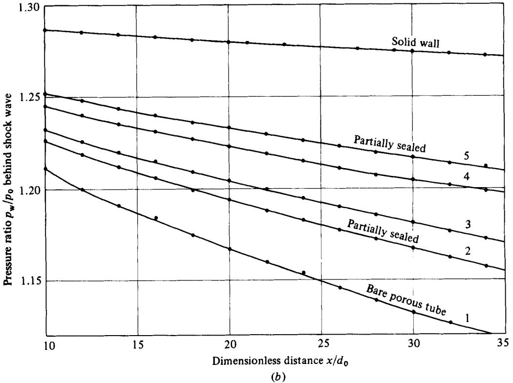
FIGURE 2. (a) Spatial decrease of pressure ratio behind shock wave for five surface configurations of a porous tube and for a tube with solid walls. (b) Spatial decrease of pressure ratio behind shock wave between  $x/d_0 = 10$  and  $x/d_0 = 35$ .
