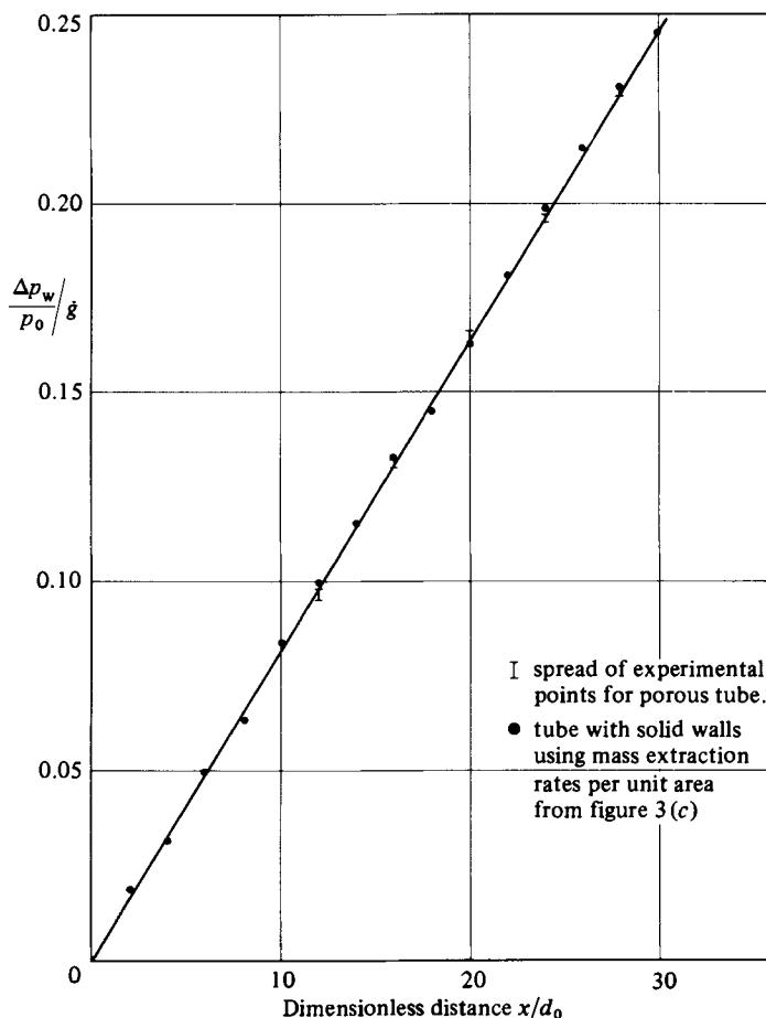
FIGURE 4. Plot of ratio  $(\Delta p_w/p_0)/\dot{g}$  for a porous tube and for a tube with solid walls using analogous values of  $\dot{g}$  from figure 3(c).
